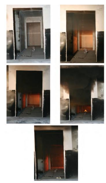
Figure A-6. Example Fire Progression from Test CRA 1
