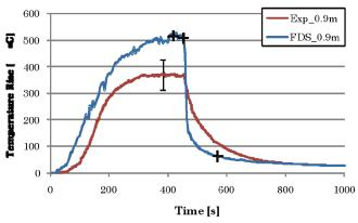
Figure 44: Measured vs. Predicted Temperature at the 0.9 m (2.9 ft) Thermocouple Location in the Burn Compartment
