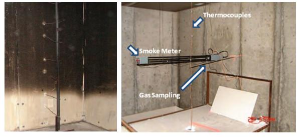
Figure C-9: Burn Room Thermocouple Array Figure C-10: Target Room Instrument Cluster
