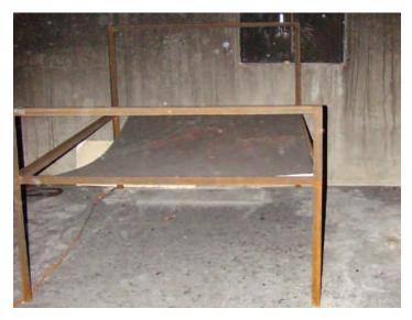
Figure 5: Noncombustible Furniture Used in the Time-to-Task Experiments
