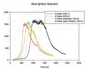
Figure A-9. HRR, Slow Ignition, Compartment Test
