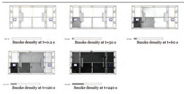
Figure B-2: Time-dependent smoke density contours in field structure with fast growth fire Page 192 of 300
