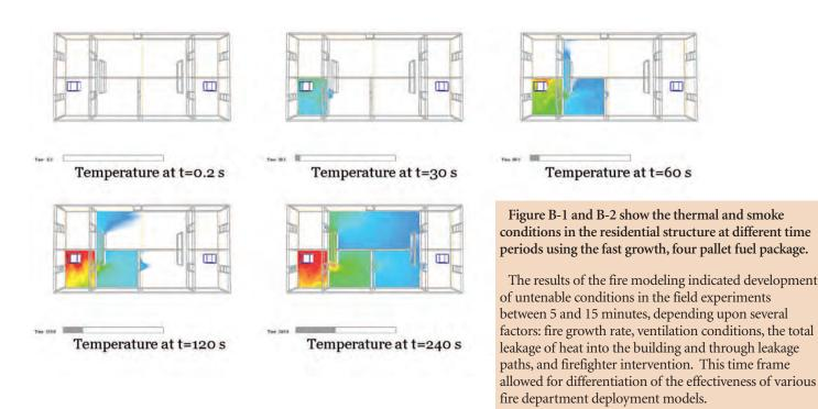
Figure B-1: Time-dependent temperature contours in field structure with fast growth fire
