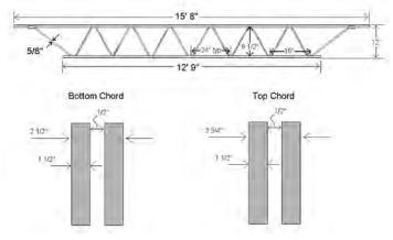
Figure C-3: Structural Steel Dimensions
