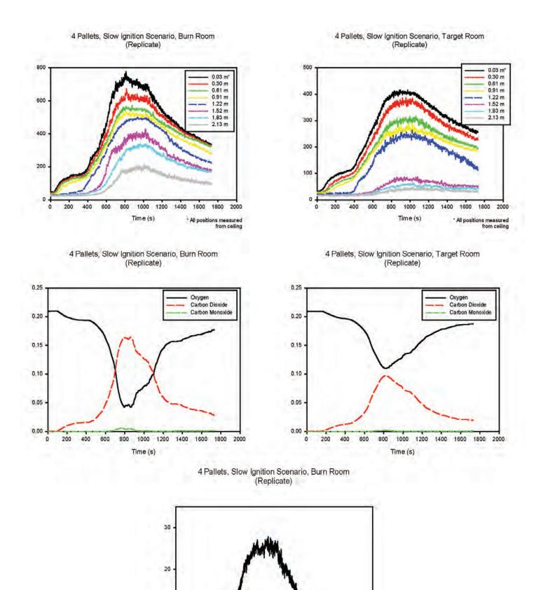
Figure A-14. Temperature, Gas Concentration, and Heat Flux During Test CRA 4, 4 Pallets, Slow Ignition Scenario (Replicate)
