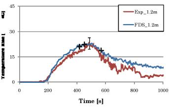
Figure 51: Measured vs. Predicted Temperature at the 1.2 m (3.9 ft) Thermocouple Location in the Bedroom
