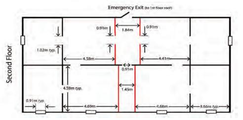
Figure C-2: Dimensions of the Burn Prop Floor Plan
