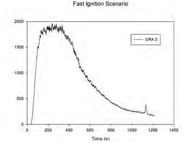
Figure A-10. HRR, Fast Ignition, Compartment Test Page 186 of 300
