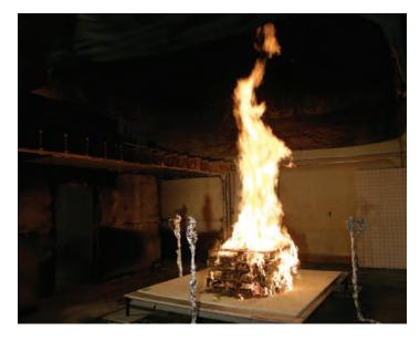
Figure 2: Test Burn of Pallets in Laboratory
